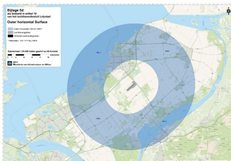
Outer horizontal surface.
